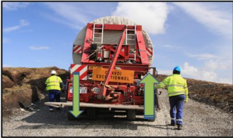
Fig. 14. Managing the effect of 2% camber on a wind farm, balancing the load.
