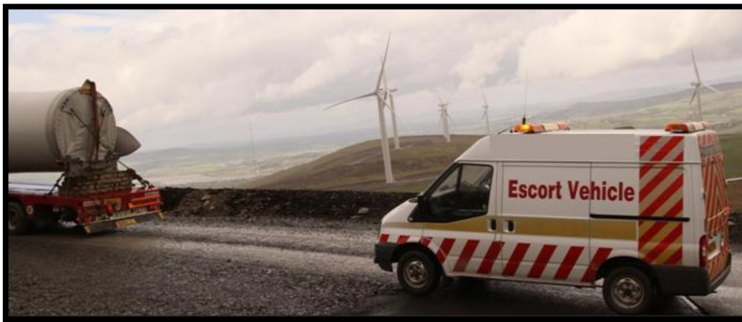
Fig. 8. Providing 'Rear vision' escort of tower section transport.
