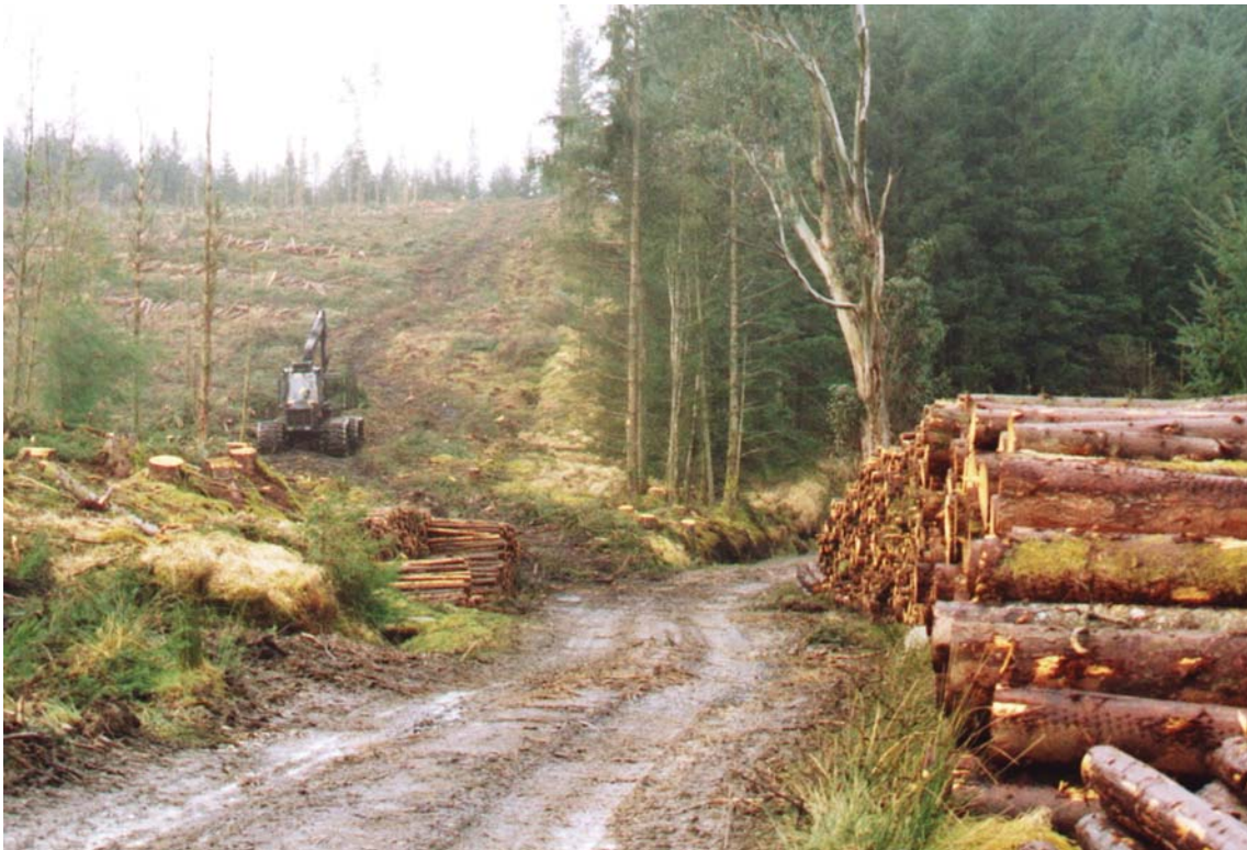
PHOTO 3: Forwarder using an extraction rack to access the forest road.
