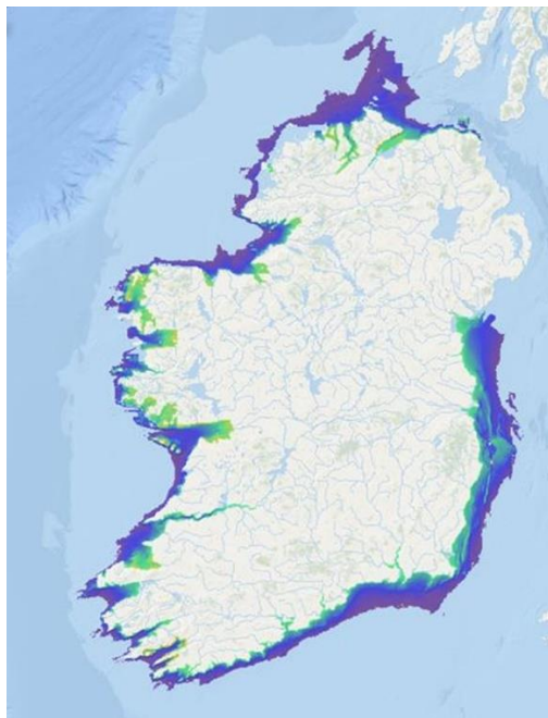
Figure 1: Extent of available seabed at water depth of 60 metres or less in Ireland's maritime area. – Source: Everoze using INFOMAR data.
