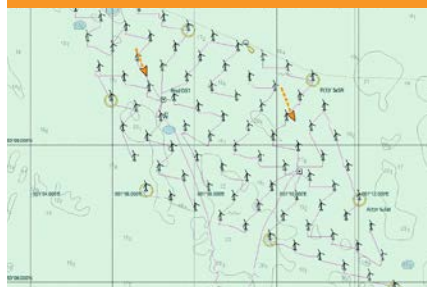
Example of a recent XOCEAN Offshore Wind survey campaign showing multiple USVs operating simultaneously
