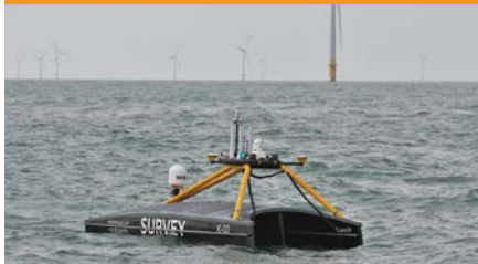
XOCEAN XO-450 performing survey operations on Greater Gabbard Offshore Wind Farm
