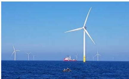
XOCEAN XO-450 performing survey operations on the Hornsea One Offshore Wind Farm
